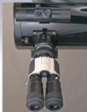
Maxbright-Bino am 8" Newton, - 2" Four-in-One-Adapter, 2" Newton-Komakorrektor 1.7x, 5 mm Hyperion-Okulare, Baader SkySurviv V Vietersucher
