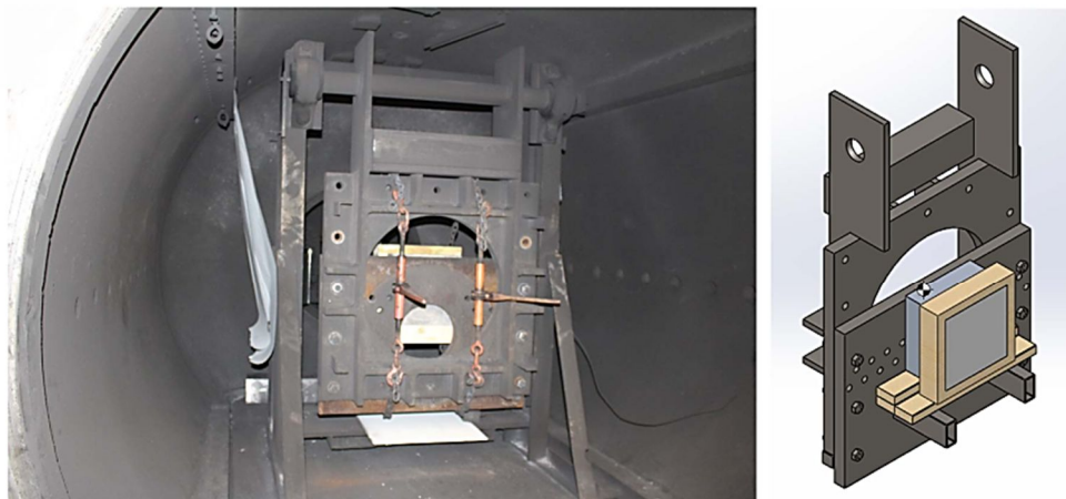
Figure 2. Photograph of the back side of the pendulum in the target vacuum chamber before the impact experiment (left). Drawing of the pendulum assembly from the front (right).
