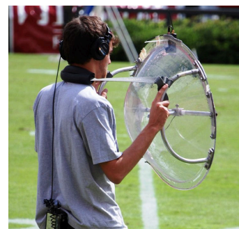
Parabolisches Mikrofon (Richtmikrofon) im Einsatz. ©: JGlover - Attribute to J. Glover, Atlanta, Georgia in any use (including derivative) outside of WikiMedia Foundation projects. - Own work, CC BY-SA 3.0, Ausschnitt, https://commons.wikimedia.org/w/index.php?curid=2896587 .
